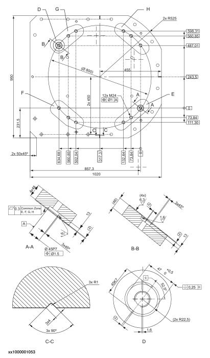
E, F, G, H Common tolerance zone (accuracy all over the base plate from one contact surface to the other)
